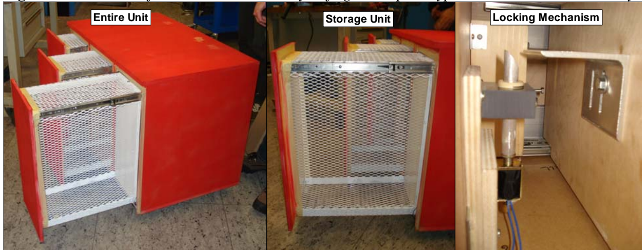
Figure 13: Pictures of the Secure Community Refrigerator prototype, taken in Berlin, Germany
