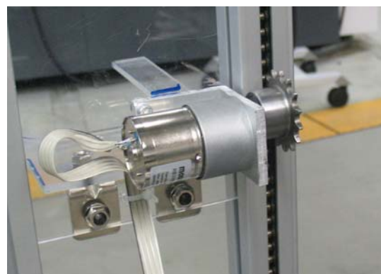
Figure 6.3 – Motor and sprocket assembly
