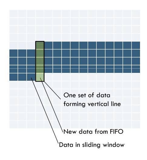
□ Revised structure with stream and sliding window
