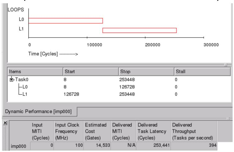
Sample result of fir filter with stream
