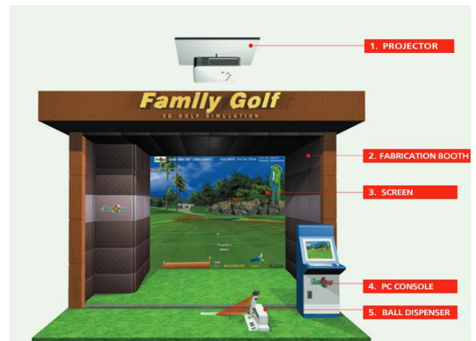
Figure 8. Configuration of screen golf machine
