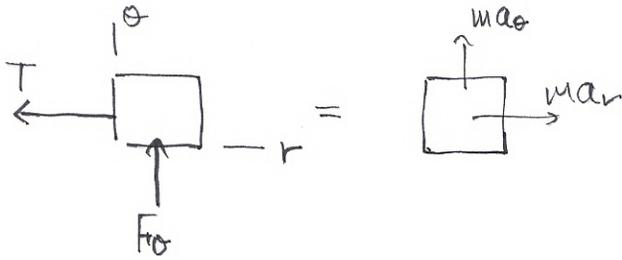
Before wire breaking  $T = -18\text{ N}$ ,  $\ddot{r} = 0$ ,  $r = 0.5\text{ m}$
