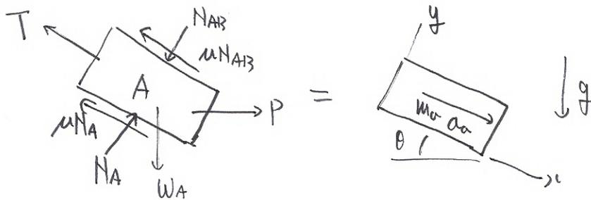
Constraint of cable:  $x_A + x_B = \text{const}$
