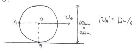
$$V_{4/6} = r_{i}w = r_{i}\frac{v_{o}}{r} = v_{o}$$
