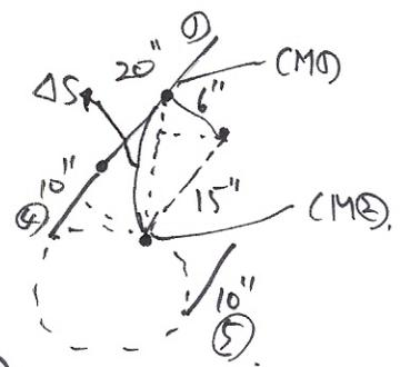
$$\Delta V_g(\text{bend})_{\textcircled{2} \rightarrow \textcircled{3}} = -0.8 \left( \frac{6}{12} \pi \right) \frac{10}{12} \sin 60^\circ = -0.907 \text{ ft} \cdot \text{lb}$$
