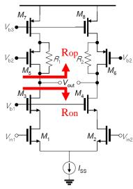
(a) Compute the differential gain of the circuit.  $R_1$  (= $R_2$ ) can have an arbitrary resistance value.
