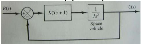
**3.** Referring to the system shown below, Determine the values of K and k such that the system has a damping ratio  $\zeta$  of 0.7 and an undamped natural frequency  $\omega_n$  of 4 rad/sec.
