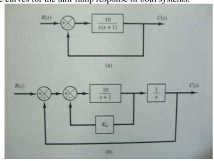
**2.** Figure shown below is a block diagram of a space-vehicle attitude-control system. Assuming the time constant T of the controller to be 3sec and the ratio of torque to inertia K/J to be  $2/9 \text{ rad}^2/\text{s}^2$ , find the damping ratio of the system.
