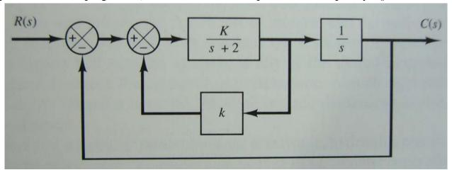
**4.** Using MATLAB, obtain the unit-step response, unit-ramp response, and unit-impulse response of the following system:
