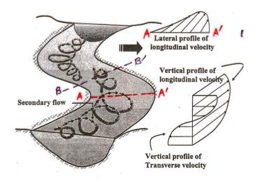
Meandering and secondary flow in open channel (Seo et al, 2005)
