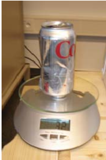
Figure 4: Image of weight scale to measure weight of empty can
