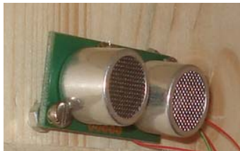
Figure 5: Image of ultrasonic wavelength sensor to count cans
