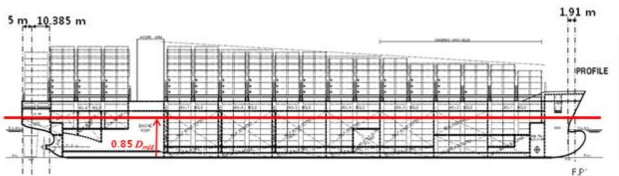
[Figure 3: General Arrangement of 7,000TEU Container ship]
