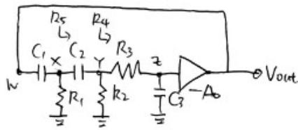
$$\frac{Z}{Y} = \frac{\frac{1}{sC_3}}{R_3 + \frac{1}{sC_3}} = \frac{1}{sC_3 R_3 + 1} = \frac{1}{sCR + 1}$$
