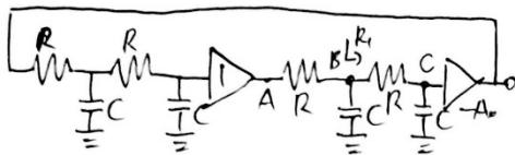
$$(a) R_1 = \frac{1}{sC} \parallel \left( R + \frac{1}{sC} \right) = \frac{\frac{1}{sC}(R + \frac{1}{sC})}{\frac{2}{sC} + R} = \frac{sCR + 1}{sC(2 + sCR)}$$
