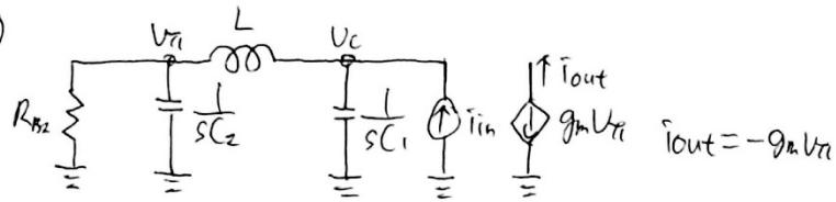
$$\left( \frac{1}{R_{B2}} + sC_2 \right) V_{pi} = \frac{V_c - V_{pi}}{sL}$$
