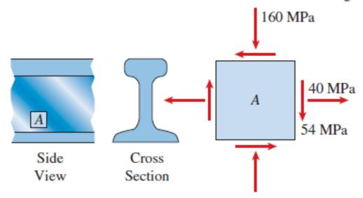
**7.2-15** An element in *plane stress* from the frame of a racing car is oriented at a known angle  $\theta$  (see figure). On this inclined element, the normal and shear stresses have the magnitudes and directions shown in the figure.
