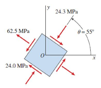
Derive below equation (Eq. 1) using plane stress conditions (Eq. 2 and 3)
