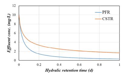
*PFR* outperforms CSTR for  $2^{nd}$  order reaction, which is the same conclusion as what we saw in the class for  $1^{st}$  order reaction.
