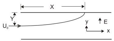
4. Consider a flow of evaporating particles in a one-dimensional (x-direction) duct. The particles evaporate according to the D<sup>2</sup>-law and are always in kinetic equilibrium with the gas. The number flow rate  $\dot{n}$  of the particles is constant so  $\dot{n} = n\tilde{v}A = n\langle u\rangle A = const$ , where *n* is the particle number density. The particle volume fraction is sufficiently small that the continuous phase volume fraction can be taken as unity,  $\alpha_c \simeq 1.0$ .
