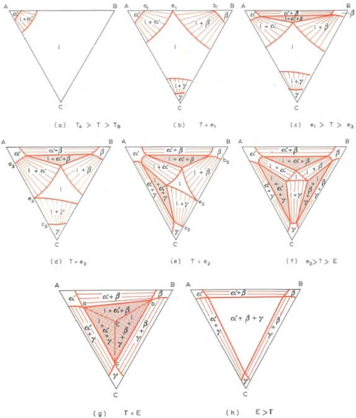
Fig. 176. Isothermal sections through the space model of Fig. 173a.
