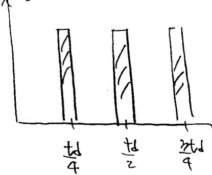
$$I_1 = I_2 = I_3 = \frac{1}{2} \times p_0 \times \frac{t_d}{2} = \frac{p_0 t_d}{4}$$
