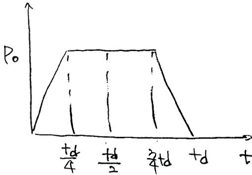
$$m\ddot{u} + ku = p(t) = \begin{cases} P_0 \frac{t}{t_d} = P_0 \frac{4t}{4t_d} & t \leq \frac{t_d}{4} \\ P_0 & \frac{t_d}{4} \leq t \leq \frac{3t_d}{4} \\ 4P_0 \left(1 - \frac{t}{t_d}\right) & \frac{3t_d}{4} \leq t \leq t_d \end{cases}$$
