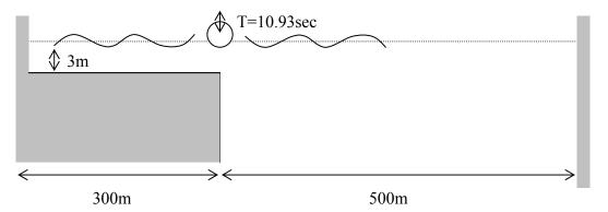
Tank depth in left domain is 3m and depth in right domain can be considered as deep water. The both sides are solid walls. There is a cylindrical wave maker just above the step of two domains, which oscillates with the period of 10.93sec.
