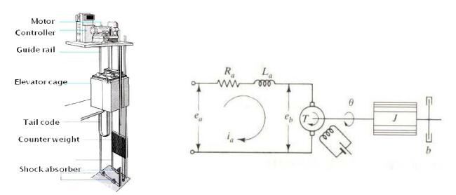
(1) Assuming that the armature inductance,  $L_a$ , is negligible, derive the equations of motion of the system.
