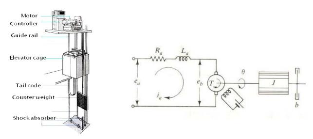
(1) Assuming that the armature inductance,  $L_{\boldsymbol{a}}$ , is negligible, derive the equations of motion of the system.
