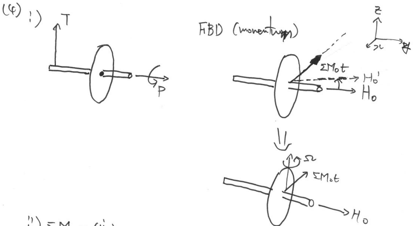
ii)  $\Sigma M_0 = (\dot{H}_0)_{Oxyz} + \Omega \times H_0$
