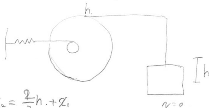
$$3 \left( \begin{array}{l} T_2 = 0 \\ V_2 = -m_A g h + \frac{1}{2} k x_2^2 \end{array} \right. \quad \left. \begin{array}{l} x_2 = \frac{2}{3} h + x_1 \\ = \frac{2}{3} h + 0.1 \end{array} \right) \rightarrow 3$$
