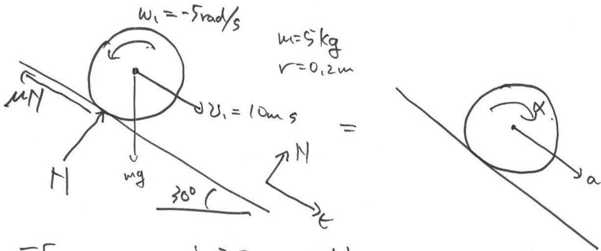
$$\Sigma F_t \Rightarrow mgs \sin 30 - \mu N = ma \quad \text{--- ①}$$
