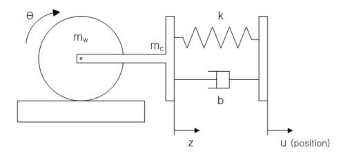
5. Given the combined translation and rotational system shown in the figure find the transfer function G(s) = X(s)/T(s)
