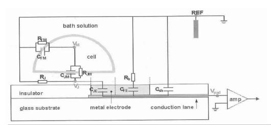
$R_{FM},\,C_{FM}\,$  : Free membrane resistance and capacitance
