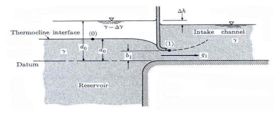
3. The two-dimensional overflow structure (dam spillway) produces the flowfield shown below. Calculate the magnitude of the horizontal component of the resultant force the water exerts on the structure when the gate is open. Compare this with the magnitude of the horizontal component of the resultant force the water exerts on the structure when the gate is closed. Assume the water is an ideal fluid. The specific weight of the water is 9,800 N/m<sup>3</sup>. (20 points)
