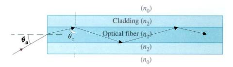
express the maximum angle of incidence  $\theta_a$  in terms of  $n_o$ ,  $n_1$ , and  $n_2$  for the rays incident on the fiber axis at the core's end face to be trapped inside the core by total internal reflection.
