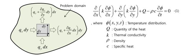
Figure 6 Problem of heat flow in a two-dimensional domain
