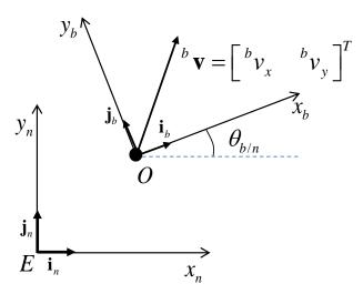
7.1. Derive the rotational transformation matrix, which can transfer the vector  ${}^{b}\mathbf{v}$  to vector  ${}^{n}\mathbf{v}$ .
