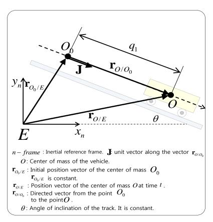
11.1. Derive the equations of motion represented by  $x_{O/E}$ ,  $y_{O/E}$  using augmented formulation.
