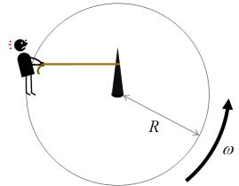
3.1. When the person is rotating with the disk, the velocity vectors have the same magnitude but they differ in direction. Because of this change of direction, the motion of the person is "accelerated motion". Derive the force exerted on the person in terms of the velocity of the person, radius of the disk R, angular velocity  $\omega$ . And describe the motion of the person in inertial reference frame.
