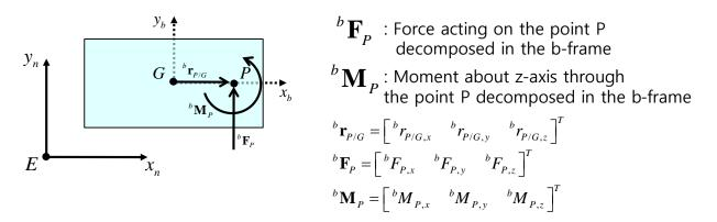
9.1. Calculate the force  ${}^{b}\mathbf{F}_{G}$  and moment  ${}^{b}\mathbf{M}_{G}$  exerted on the point G in force equilibrium system. (Calculate the components of the each vector)
