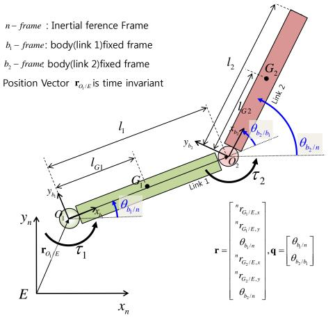
Mass and mass moment of inertia about point  $G_1$  of link 1:  $m_1$ ,  $I_1$ Mass and mass moment of inertia about point  $G_2$  of link 2:  $m_2$ ,  $I_2$
