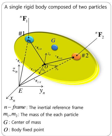
The equations of motion for this single rigid body are as follows: - Force equation
