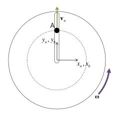
n-frame: inertial frame b-frame: body-fixed frame
