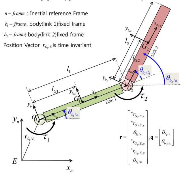
Mass and mass moment of inertia about  $z_{\rm G1}$ -axis through point  $G_1$  of link 1:  $m_1$ ,  $I_1$  Mass and mass moment of inertia about  $z_{\rm G2}$ -axis through point  $G_2$  of link 2:  $m_2$ ,  $I_2$
