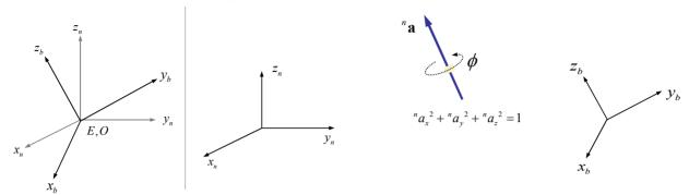
$$\mathbf{R}_{\mathbf{a},\phi} = \begin{bmatrix} (1-\cos\phi)^n a_x^2 + \cos\phi & (1-\cos\phi)^n a_x^n a_y - {}^n a_z \sin\phi & (1-\cos\phi)^n a_z^n a_x + {}^n a_y \sin\phi \\ (1-\cos\phi)^n a_x^n a_y + {}^n a_z \sin\phi & (1-\cos\phi)^n a_y^2 + \cos\phi & (1-\cos\phi)^n a_y^n a_z - {}^n a_x \sin\phi \\ (1-\cos\phi)^n a_z^n a_x - {}^n a_y \sin\phi & (1-\cos\phi)^n a_y^n a_z + {}^n a_x \sin\phi & (1-\cos\phi)^n a_z^2 + \cos\phi \end{bmatrix}$$
