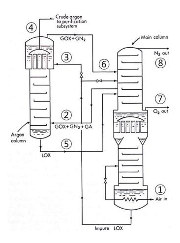
Right: air-separation double-column system, Left: argon recovery subsystem
