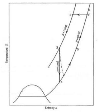
(3) (3p)If the regenerator were less than 100 percent effective, the temperature of the gas leaving the regenerator at point 3 in Fig. 5.21 would be somewhat higher than ideal. This means that some of the energy that could have been absorbed from the low-temperature region.
