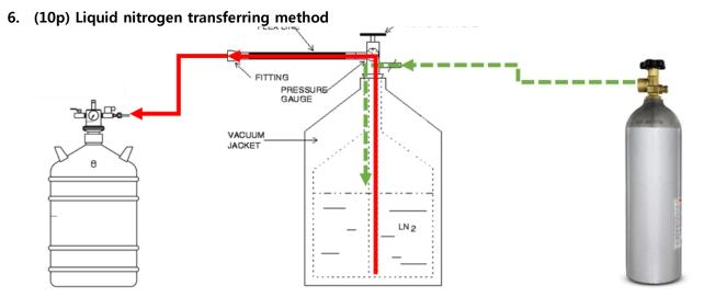
(5p)Tube connection is seen in above schematic diagram. The compressed nitrogen gas is injected into the nitrogen supply tank. (5p)High pressure gas push the liquid nitrogen to get out of the supply tank and it is transferred to the small Dewar.
