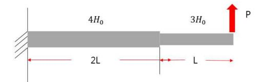
(1) Construct the stiffness matrix of the beam (15 pts)
