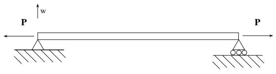
Length = L, Flexural stiffness = EI (const.), Mass/length = m (const.), Area = A (const.)
