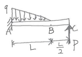
(4) With the calculated vertical force of P from above question of (3), determine the new angle of rotation  $\theta_{\rm C}$  at the point of C.
