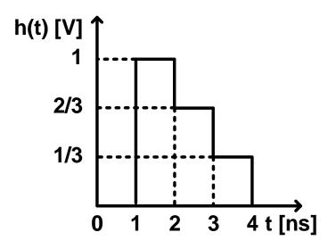
A. Draw a single-bit response (1-bit, 1V-rectangular pulse) of a 1-Gbps NRZ transmission. (5 points)
