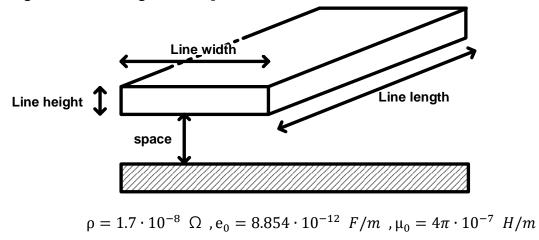
A. What is its capacitance, DC resistance, inductance per meter? (5 points)
