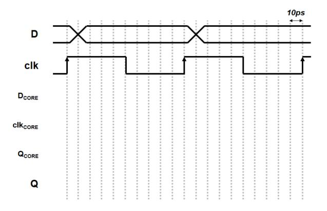
(b) Draw the curve of  $T_{CQ}$  (clk-to-Q delay) vs.  $T_{D-clk}$ . (Note that  $T_{D-clk}$  is the time difference between the transitions of  $D_{CORE}$  and clk<sub>CORE</sub>.) (5 points)
