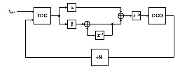
a. Determine  $\alpha$  and  $\beta$  which make the ADPLL have the open-loop bandwidth of 10 MHz and the phase margin of 60°. Assume  $z^{-D} = z^{-0}$ .
