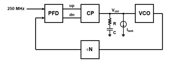
a. Determine loop filter parameters R and C that realize the loop bandwidth of 10 MHz and the damping factor  $\zeta$  of 0.7. Assume  $I_{leak} = 0$ .
