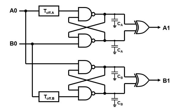
a. Draw the waveform of B1. Assume that  $T_{off,B} = T_{off,A} = T_{off}$  and  $C_B = C_A = C$ . Also assume that the trans-conductance of the NAND output is  $g_m$  at the metastable state.
