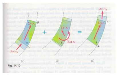
Auxiliary system of particles remaining constant for  $\Delta t$
