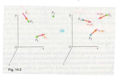
Eq (14.3): The system of the internal forces  $\overline{f_{ij}}$  is equipollent to zero. It does not mean that the internal forces have no effect on the particles.
