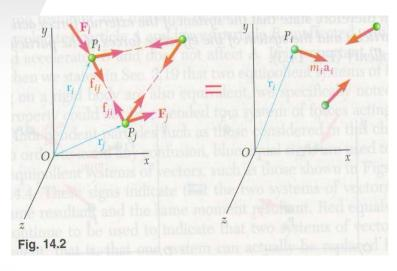
Internal force  $\overrightarrow{f_{ij}}$ : according to Newton's 3<sup>rd</sup> law,  $\overrightarrow{f_{ij}}$  and  $\overrightarrow{f_{ji}}$  are equal and opposite, and have the same line of action.
