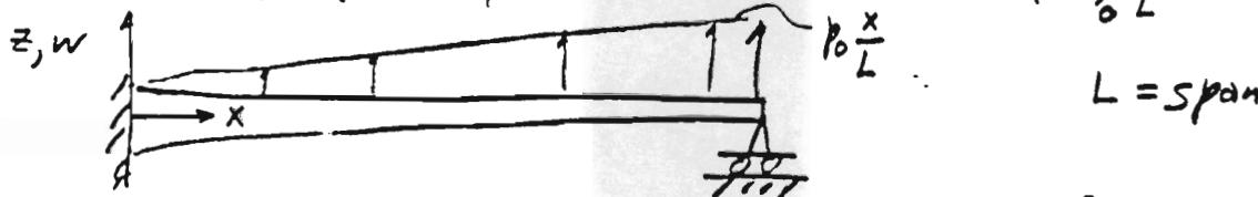
$$\text{Assume: } w(x) = \alpha_1 + \alpha_2 \frac{x}{L} + \alpha_3 \left( \frac{x}{L} \right)^2 + \alpha_4 \left( \frac{x}{L} \right)^3$$
