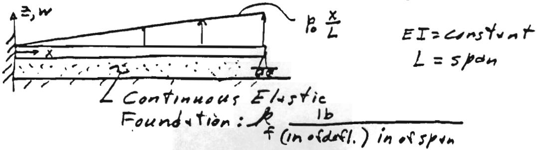
$$U = \int_0^L \frac{EI}{2} \left( \frac{d^2w}{dx^2} \right)^2 dx + \int_0^L \frac{k_f}{2} [w(x)]^2 dx$$
