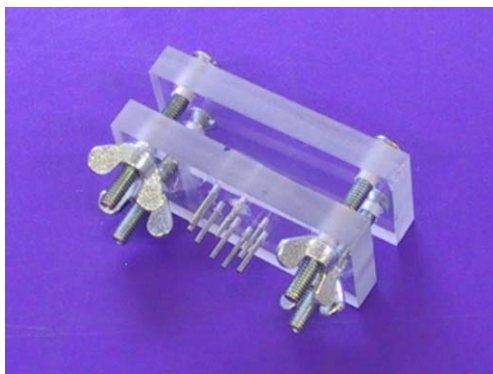
Figure 20: Device to seal flow cell by pressure
