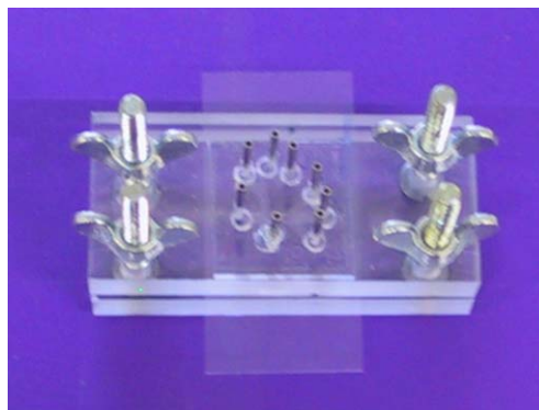
Figure 21: Pressure device with installed flow cell
