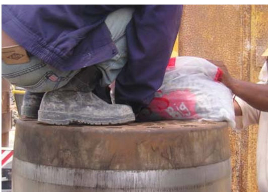
Figure 5. Loading of Statnamic fuel
