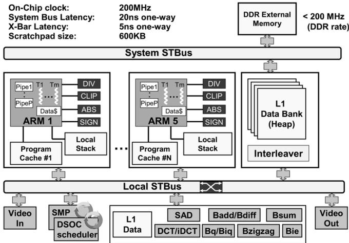
Fig. 6. Target MPEG4 video encoder MP-SoC.
