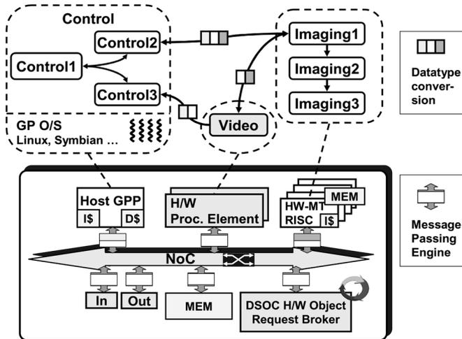
Fig. 2. DSOC model to platform mapping.
