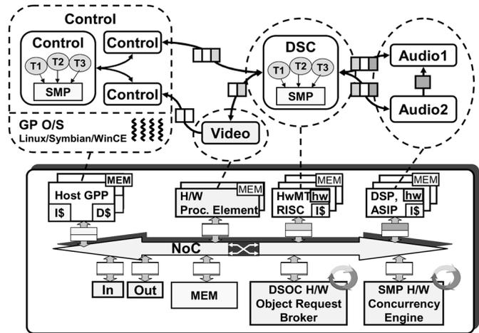
Fig. 3. Mixed DSOC-SMP model to platform mapping.
