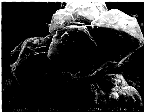
Fig. 5. SEM microstructure showing the evolution of diamond over soot on the iron substrate beneath which quartz was placed. The other deposition conditions were the same as those of Fig. 3.
