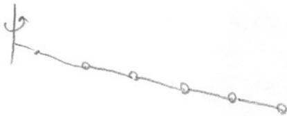
1-D finite element representation of the blade
