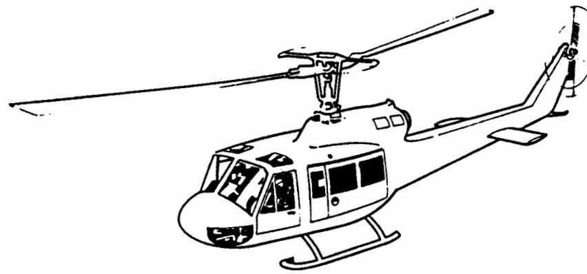
Figure 1-2 A two-bladed single main rotor helicopter
