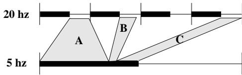
Figure 11: Interleaving of Rate Group Thread Execution
