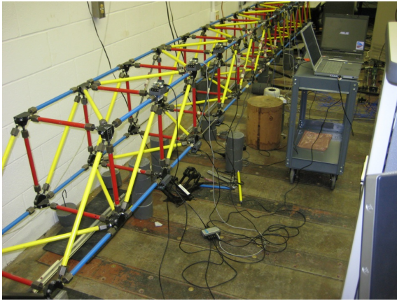
Figure 10. 3D truss test structure
