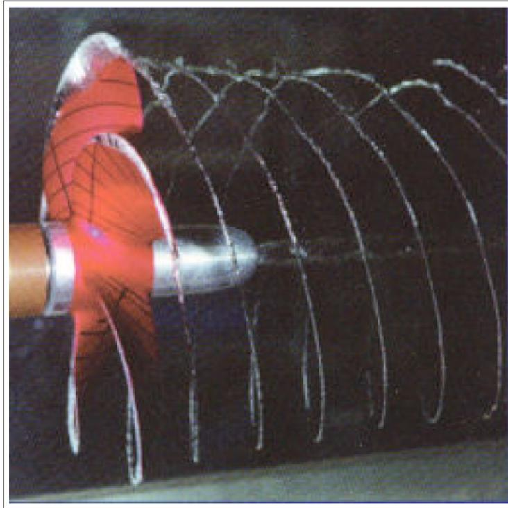
**Figure 6.3** Tip vortex cavitation of a marine propeller.
