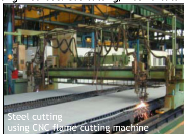
Steel cutting using CNC plasma cutting machine
