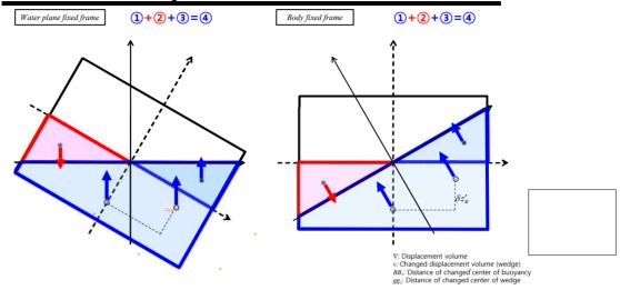
The moments described in the water plane fixed reference frame can be described in the body fixed reference frame by decomposing the forces and moment arms in the body fixed reference frame.
