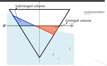
For the ship to be in static equilibrium, the buoyant force and gravitational force have to be on one line, so that the total moment about the transverse axis through any point becomes 0:
