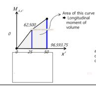
After finding each longitudinal moment of the sectional area about the x'  $axis(\mathcal{M}_{A,x})$ , the <u>longitudinal moment of the displaced volume</u> can be obtained by integration of the transverse moment of the sectional area over the length of ship.
