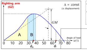
Area A: Area under the righting arm curve between the heel angle of  $0^\circ$  and  $30^\circ$ Area B: Area under the righting arm curve between the heel angle of  $30^\circ$  and  $\min(40^\circ, \phi_f)$   $\divideontimes \phi_f$ : Heel angle at which openings in the hull  $\phi_m$ : Heel angle of maximum righting arm
