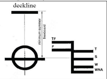
The Plimsoll<sup>1)</sup> mark or Freeboard Mark is a symbol indicating the of the ship in the water, leaving a minimal freeboard for safety. The freeboard is marked according to the result of the freeboard calculation, where the summer freeboard in salt water ( $d_s$ ) is established.
