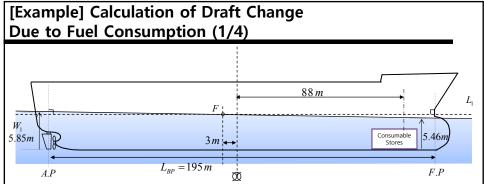
During a voyage, a cargo ship uses up 320ton of consumable stores (H.F.O: Heavy Fuel Oil), located 88m forward of the midships.
